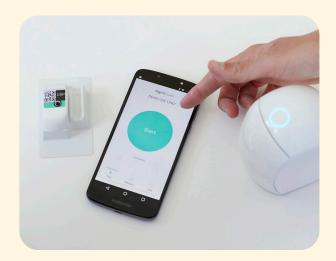
The Egoo device is small, fist sized, and portable. The tests can be made from either blood, plasma or mouth swab depending on the specific test and takes 5-30 minutes for most tests. Results are qualitative on par with existing laboratory tests. The tests are run from either smartphone or laptop and the results shown instanteniously. It is optional to share data with a GP, hospital or other caregiver - in accordance with GDPR regulation.
