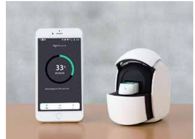
The Egoo device is small, fist sized, and portable. The tests can be made from either blood, plasma or mouth swab depending on the specific test and takes 5-20 minutes for most tests. Results are qualitative on par with existing laboratory tests. The tests are run from either smartphone or laptop and the results shown instantaneously. It is optional to share data with a GP, hospital or other caregiver – in accordance with GDPR regulation.
